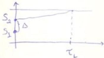
$$\begin{aligned} \Delta &= S_2 - S_1 \\ S &= S_1 & \tau &= \tau_L \\ S &= S_2 & z &= \tau_L + \Delta \end{aligned}$$
